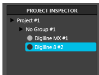
Digiline MX in DISCONNECTED state and Digiline 8,(created from the library), and not associated with any physical device
